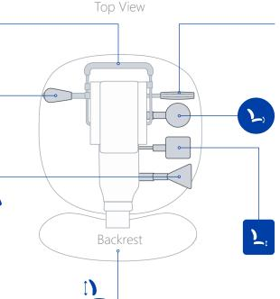
**FORWARD TILT:** To adjust the amount of forward tilt, pull up on the **CIRCULAR** paddle then tilt the seat pan slightly backward and turn this knob clockwise to increase the forward tilt position of the seat and counter clockwise to decrease the amount of forward tilt.
